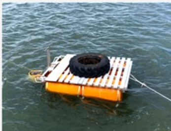
Figure 2: "Seabin mounted to a pontoon and anchored down to a fixed location at the University of the South Pacific, Marine Studies campus jetty". Source: Paris, Kwaaga, & Chintaka (2022).
